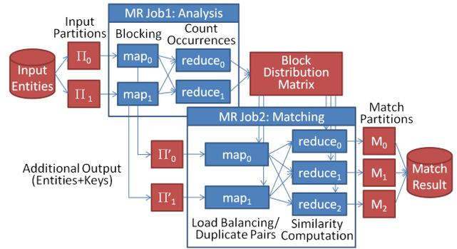
Figure 3: General scheme of Dedoop's efficient cluster utilization.
