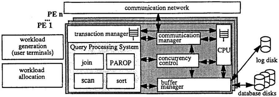
Figure 1: Gross structure of the simulation system.
