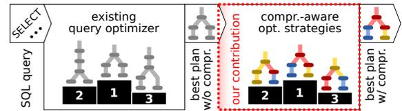
Figure 3: Compression-aware query optimization. Colors in the query plans stand for different compressed formats; grey stands for uncompressed data.
