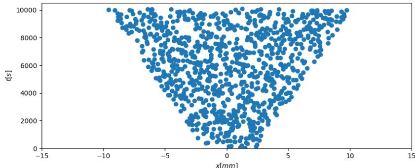
Figure 2: **Domain of heat source** - Area of laser exposure, shape of the pyramid component can be seen over the time
