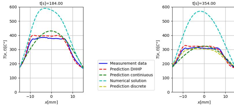
Figure 5: **Comparison of temperature prediction 3** - cooling down after exposure INC718 Left: Prediction of different models at time  $t = 184s$  Right: Prediction of different models at time  $t = 354s$
