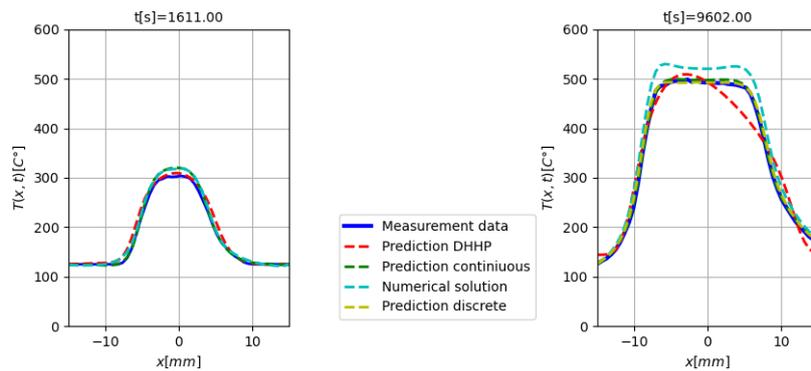
Figure 4: **Comparison of temperature prediction 2** - heating up layer by layer INC718 Left: Prediction of different models at time  $t = 1611s$  Right: Prediction of different models at time  $t = 9602s$
