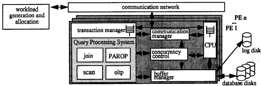
Fig. 3: Gross structure of the simulation system
