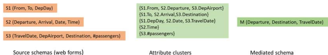
Fig. 1: Integration of web forms (query interfaces) into a mediated schema for flight bookings
