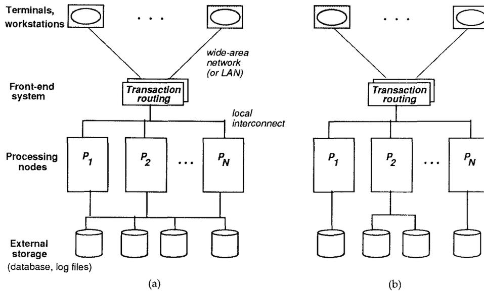
Fig. 1. DB-sharing versus DB-partitioning (a) DB-sharing (b) DB-partitioning.
