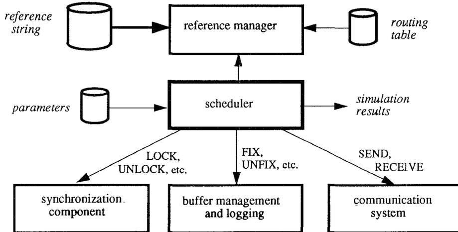
Fig. 3. Gross structure of the simulation system.
