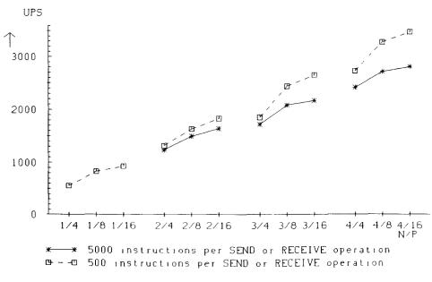
Fig. 9 Influence of communication costs on throughput (Mix 2, PCL).
