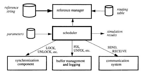
Fig. 3. Gross structure of the simulation system.
