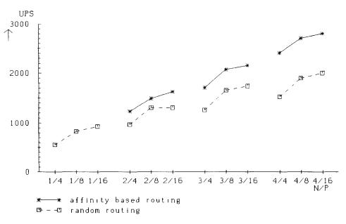
Fig. 8. Throughput for M1x 2 and PCL under different routing strategies.
