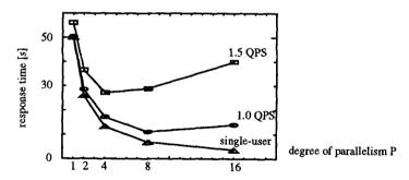
Fig. 7: Degree of parallelism vs. arrival rate (n=16, D=64)
