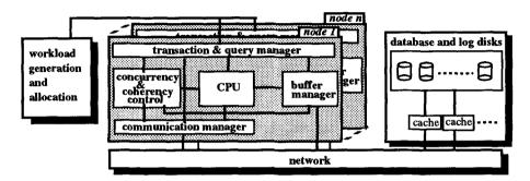
Fig. 2: Structure of the simulation system
