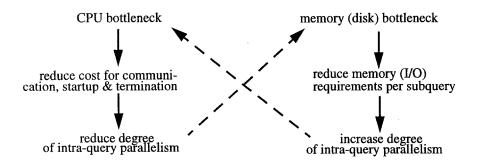
Figure 5: Tradeoffs in dynamic load balancing with multiple bottlenecks
