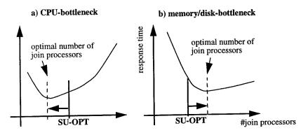
Figure 4: Optimal number of join processors in multi-user mode
