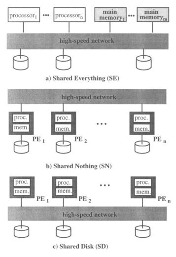
Figure 1: Architecture of parallel database systems
