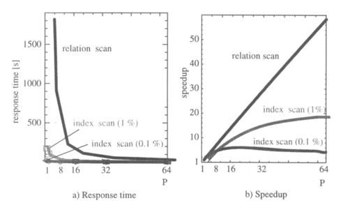
Figure 2: Parallel scan processing in SN systems (single-user mode)
