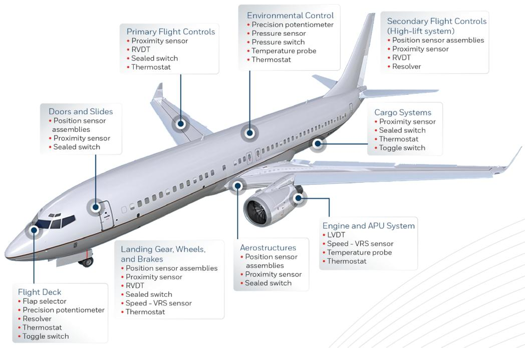
**Figure 6.1:** Sensors of an airplane [92].
