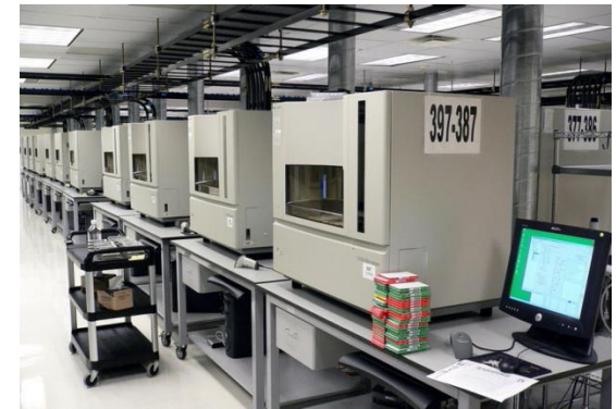
A row of DNA sequencing machines (3730xl DNA Analyzer machines from Applied Biosystems). Flickr user jurvetson: http://www.flickr.com/photos/jurvetson/57080968/
